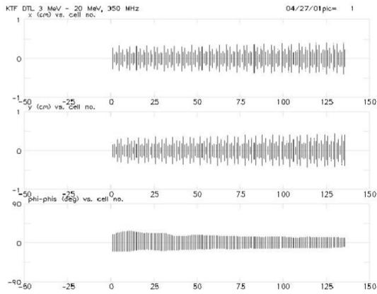
Figure 8: Beam trajectory in DTL
