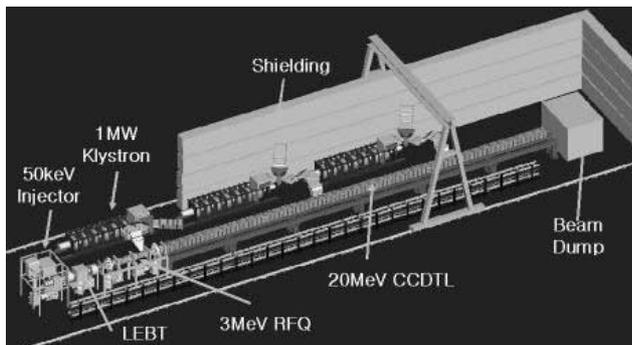
Figure 1: KTF Accelerator Plan
