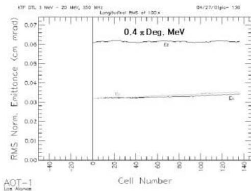
Figure 9: Emittance in DTL
