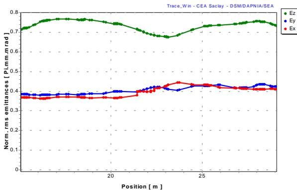
figure 8 : RMS emittance evolution of the H<sup>+</sup> beam in the funnel line.
