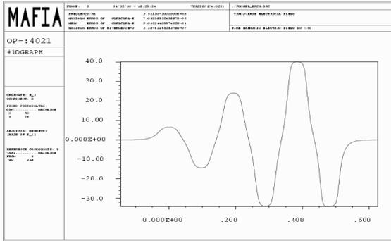
Figure 3: The transverse electrical field in the TE211 and TE111 mode structures.
