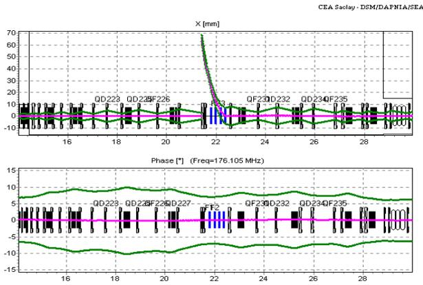
figure 6 : H<sup>+</sup> beam X and phase envelopes. A (66.5mm; 10°) frame change is applied at QuaDev entrance.
