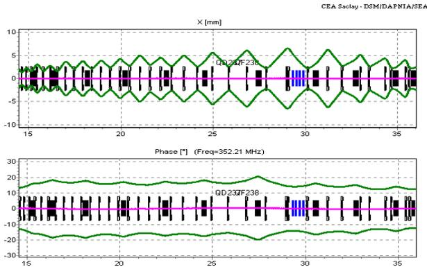
figure 7 : H<sup>+</sup> beam X and phase envelopes.
