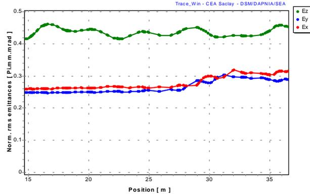
figure 9 : RMS emittance evolution of the H<sup>+</sup> beam in the funnel line.
