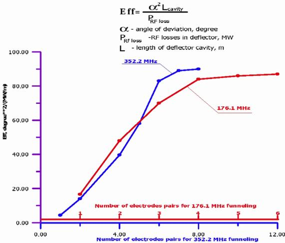
Figure 4: The efficiency of the funnel device versus the gaps number.
