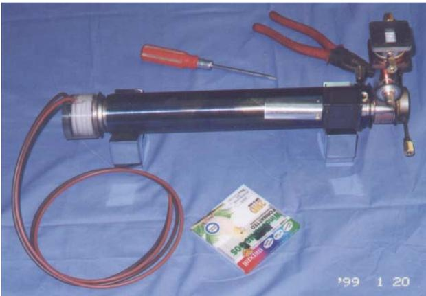
Figure 4: 6 MeV On-axis SW Guide Brazed Assembly.
