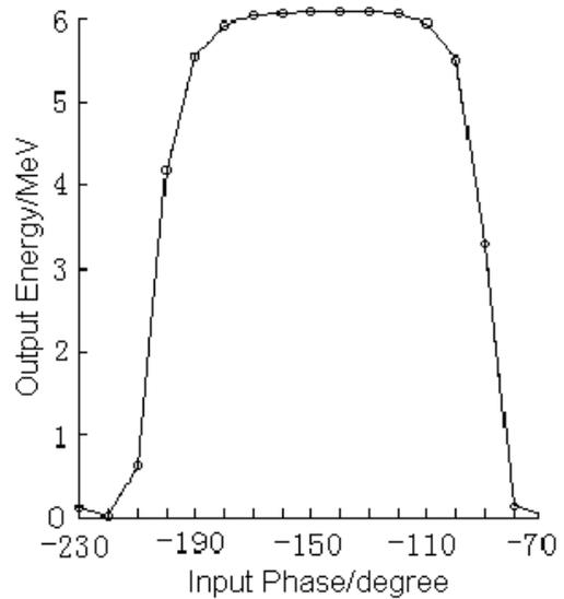
Figure 3: Energy Spectra as a Function of Input Phase.
