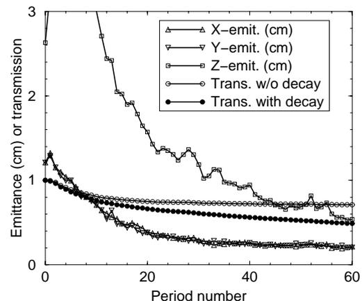
Figure 5: Beam emittance and transmission at the cooling.
