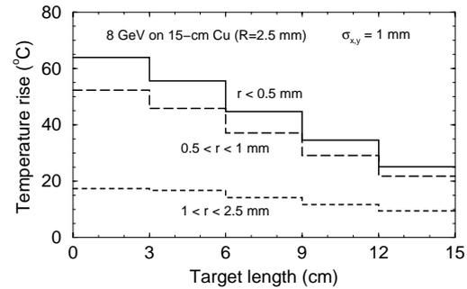
Figure 6: Instantaneous temperature rise in 2.5 mm radius copper target irradiated by a 8 GeV beam of  $5 \times 10^{12}$  ppp.
