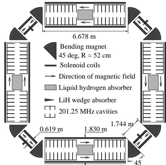
Figure 1: Layout of the ring cooler.
