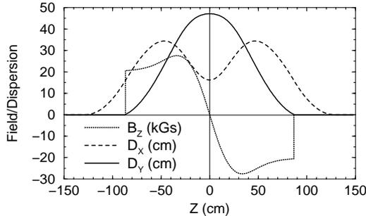
Figure 3: Axial field and dispersion functions in short SS.
