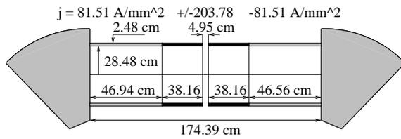
Figure 2: Layout of the short straight section.
