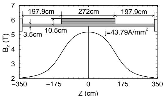
Figure 4: Layout and axial field in the long SS.
