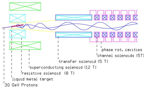
Figure 3: Shows the front end for a neutrino Factory: a proton beam hitting the target, through capture solenoid channel.
