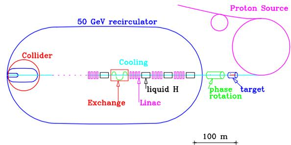
Figure 1: Schematic of How the solenoid and wedges are used in an accelerator and the other components,[4].
