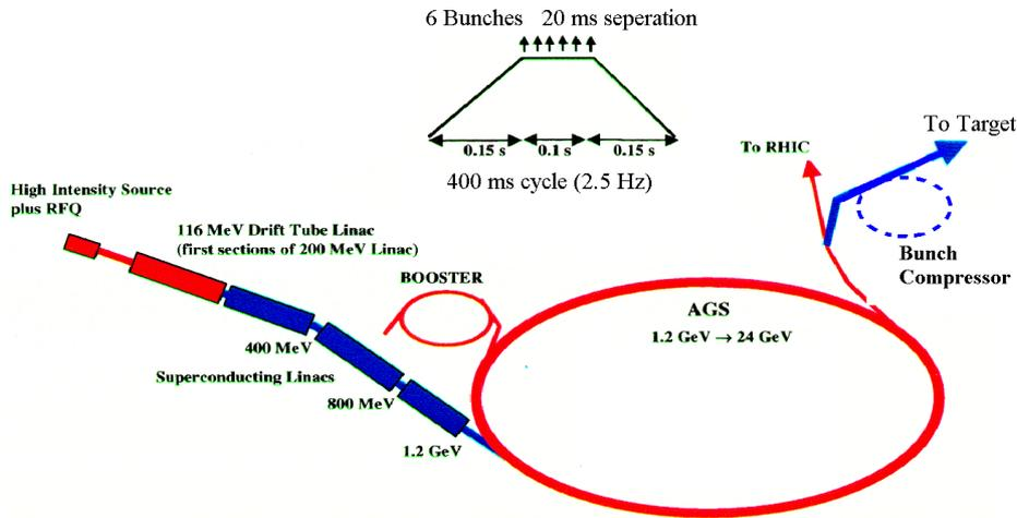
Figure 4: AGS proton driver layout. Where the Booster is replaced by Superconducting Linacs
