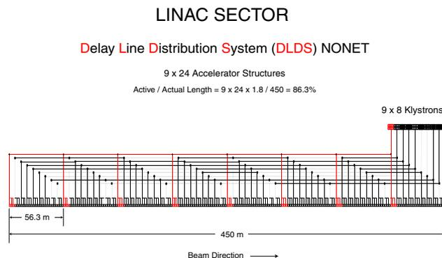
Figure 1: Schematic of rf power distribution from 8-packs to X-band structures for a typical NLC main linac sector.
