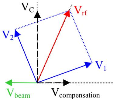
Figure 2. A schematic of  $\Delta T$  beam loading compensation.
