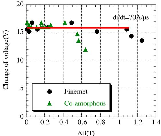
Figure 7: Voltage change versus magnetization
