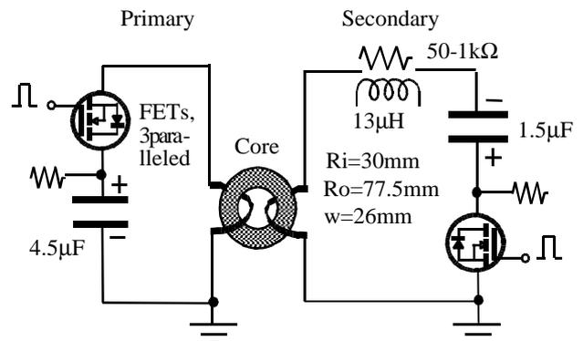
Figure 3: Equivalent circuit of experimental set up
