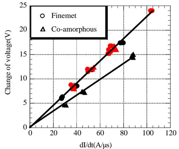
Figure 8: Voltage change dependence on  $dI/dt$
