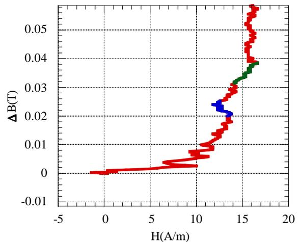
Figure 6: Typical B-H curve for short pulse loading
