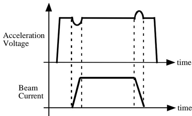
Figure 1: Schematic illustration of beam loading
