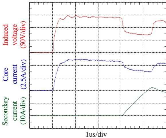
Figure 4: Typical waveform for long pulse loading
