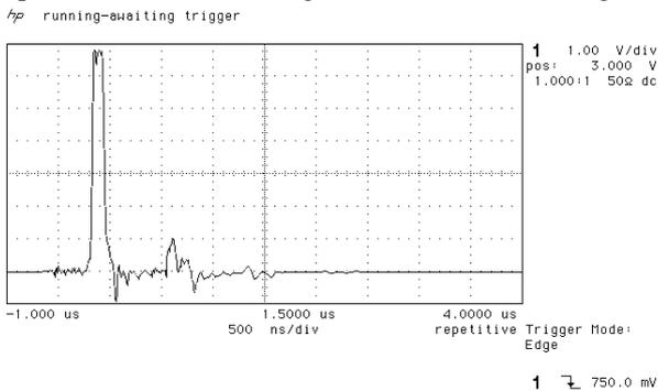
Figure 6: All-ferrite magnet with 25 Ω load @ 38 kV
