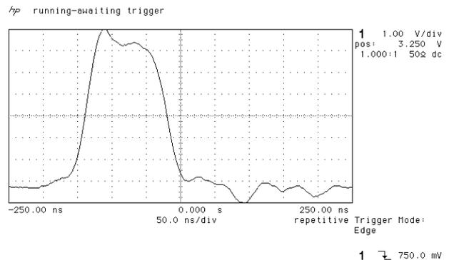
Figure 3: Current in the load of a dielectric kicker (30 kV into 16  $\Omega$ ; scale 200A/V).
