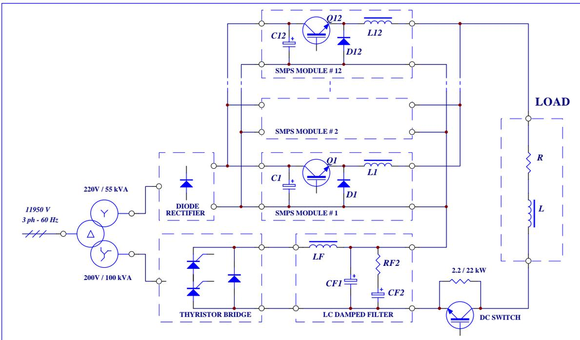
Figure 3: Basic configuration of the booster dipole power supply.
