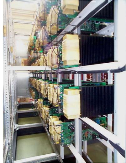
Fig 4 Modules inside the Thomcast HVPC
