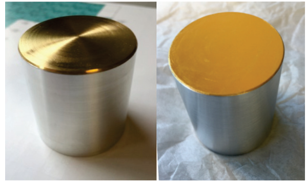
Figure 11: Example of two test targets; left: explosion bonded gold on aluminum; right: electro-plated gold on aluminum.
