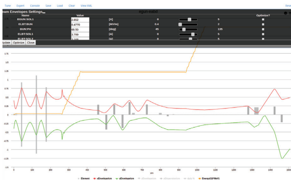
Figure 2: Screen capture of TRANSOPTR web-GUI (URL: http://hlweb.triumf.ca/beam/envelope/ ). The simulation starts near rest on the e-gun grid, and goes through two accelerating cryomodules. The turnaround time for an individual calculation is so rapid (25 ms) that the envelopes are seen to change continuously as the sliders (in the top grey box) are moved. The check boxes on the right of the slider flag those elements that are adjusted by the optimizer routines. Optimization objectives are built into the beamline's description.
