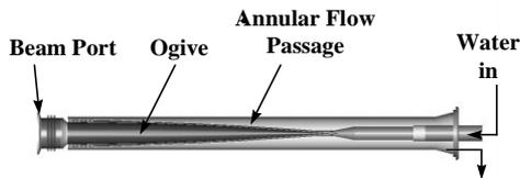
Figure 2: Ogive Beamstop Cartridge
