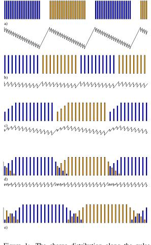
Figure 1: The charge distribution along the pulse—in case a) different trains are shown in different tones, in the other cases different half-trains are shown different tones. The number of bunches on the flat top is constant but different from the real value. The curves indicate the variation of the energy gain. Depending on the injector, a distribution in the range of d) to e) will be chosen.
