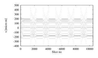
Figure 3: The final slice position for detuned structures with Q = 100. Each bunch is cut longitudinally into 21 slices, the first 500 bunches are plotted. The horizontal lines visible, are formed by equivalent slices of successive bunches. The slices of each bunch are filling the space between the minimum and maximum position.
