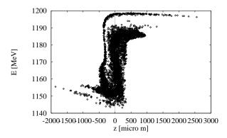
Figure 2: The phase space distribution of the particles after the last compression step in case 4. The particles represent different charges.
