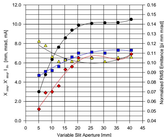
Figure 5. Beam parameters vs. Variable aperture opening. (●) Ion current; (■) rms beam size; (▲) rms divergence; (◆) normalized rms emittance. Solenoid current = 160 A.
