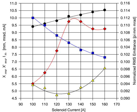
Figure 4. Beam parameters vs. Solenoid current. (●) Ion current; (■) rms beam size; (▲) rms divergence; (◆) normalized rms emittance. Variable aperture = 40 x 40 mm<sup>2</sup>.
