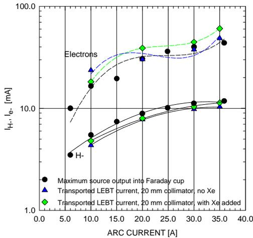
Figure 3. Ion and electron current vs. Arc current. (●) Extraction directly into faraday cup. Transported LEBT current with: (▲) residual H<sub>2</sub>; (◆) Xe gas added to LEBT. Solenoid current = 160 A. Beam energy = 40 kV.
