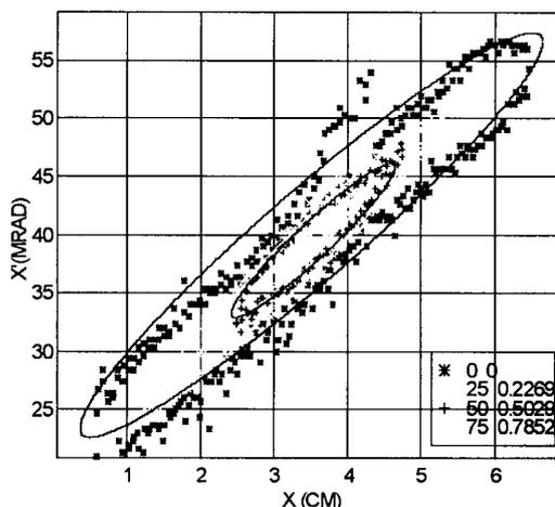
Figure 6. H- phase space at the tandem accelerator entrance plane. I(H-) = 10.5 mA, Normalized rms emittance = 0.10 π mm mrad.
