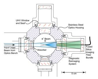
Figure 2.Central cross section of IP Optics. The parallel laser beam ( $z_R$ >> 20m) enters at right or from underneath with a  $\sigma_{in}$  of about 2.5mm. The four 8mm thick UHV seal windows with their weld rings are placed on each side of the IP, with the precision optics installed inside the vacuum chamber. 1% of the light is transmitted and reimaged on the far side of the IP for diagnostic purposes.
