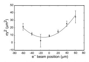
Figure 5. A typical laser-waist scan. The plot shows the measured  $\sigma_v^2$  vs e- beam x position. A parabola is used for a fit.
