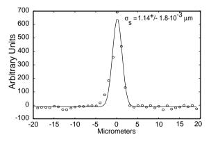
Figure 4. A typical profile monitor scan showing  $\sigma_{sy}$ . The horizontal scale is determined using the transfer matrix (R<sub>34</sub>) for the scan coils to the laser IP. The collision signal in this case is detected using the SLD polarimeter degraded e- detector, located after the first large bend in the outgoing beamline. Each data point is the average of 3 beam pulses with the laser on, with the average of 6 pulses with the laser off subtracted.
