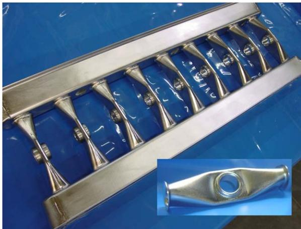
Figure 5: Some of the niobium parts of the s.c. CH-cavity which is in the final stage of production.
