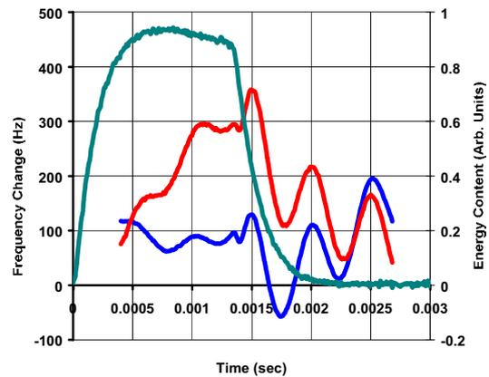
Figure 3. Lorentz force compensation at SNS cavity
