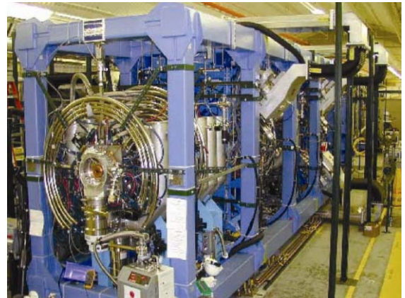
Figure 7: View of the LEDA RFQ after installation
