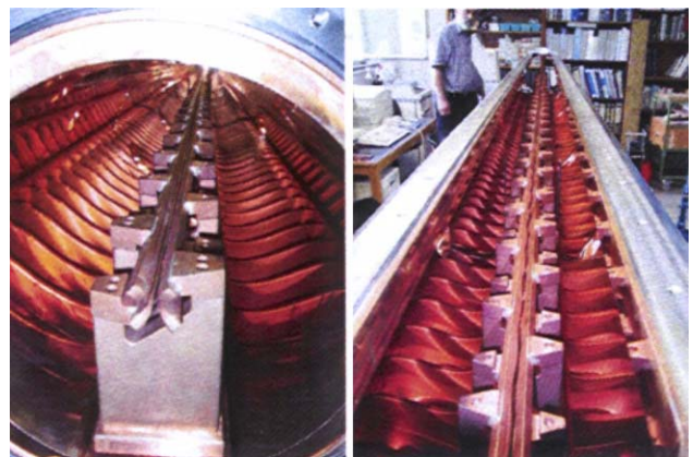
Figure 17: View of the 4 MeV 4 Rod-RFQ
