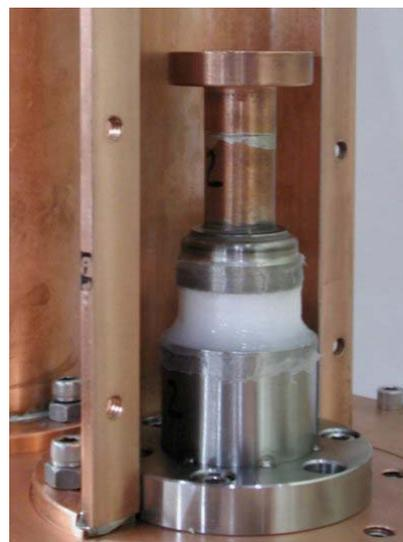
Figure 4: Modified feedthrough with shield
