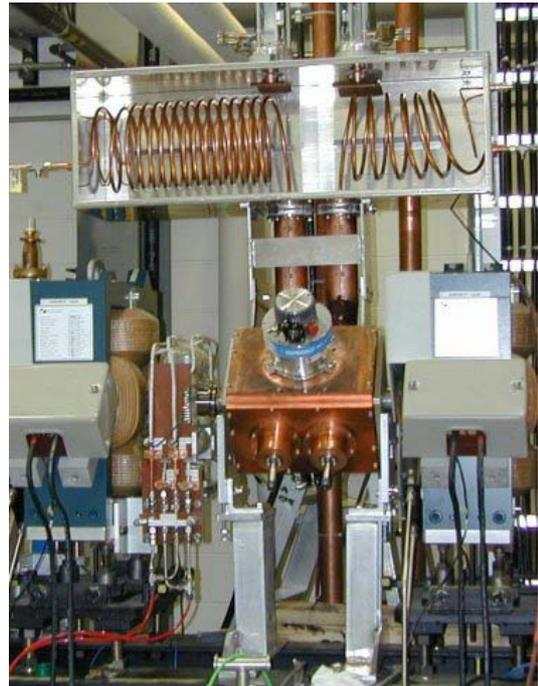
Figure 1: Photograph of dual mode chopper.
