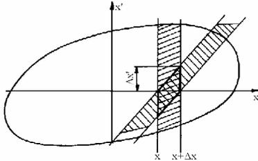
Fig.3. Element of phase volume projection on axis  $XX'$
