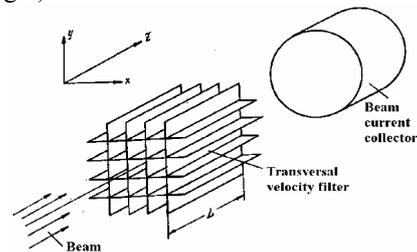
Fig.2. Schematic view of measurements.
