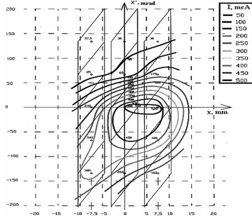
Fig.7. Lines of equal current at phase plane XX'
