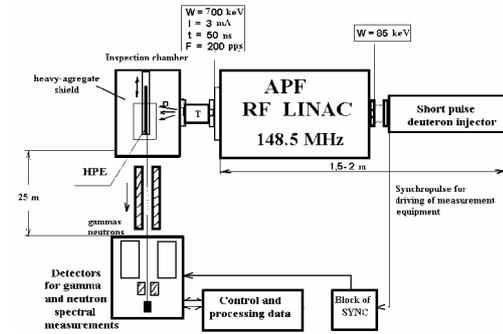
Fig.1. Functional scheme of measurement complex for HPE inspection
