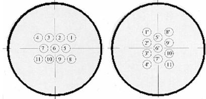
Fig.6. Configuration of beam collectors (Faraday cups) at various positions of MCS channels
