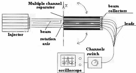
Fig.5. Scheme of beam emittance measurements.
