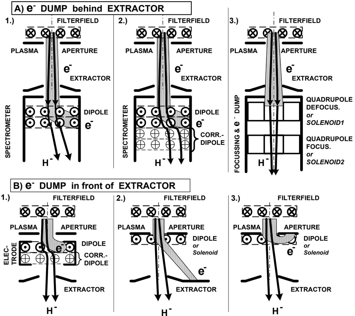
Figure 4: Configurations for dumping  $e^-$
