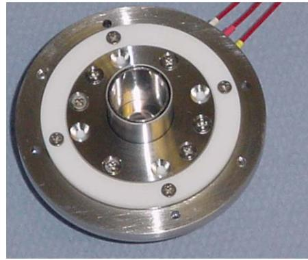
Figure 3: Insulated collar with steering
