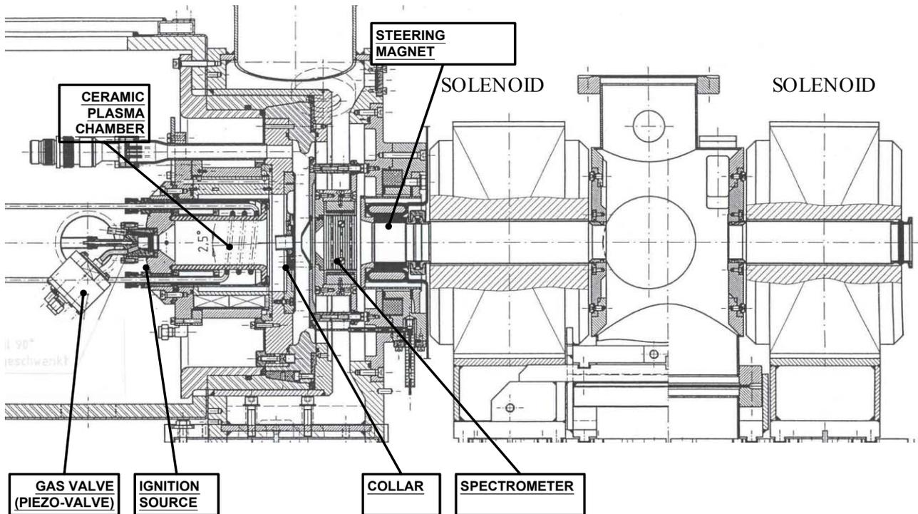
Figure 1: Source set up.
