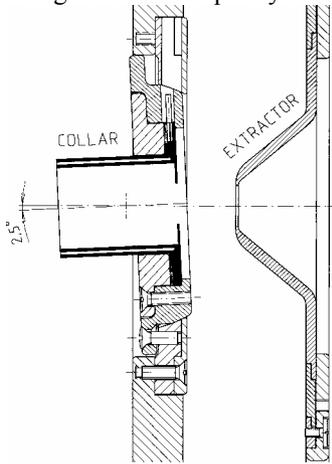
Figure 2: Collar steering and extractor
