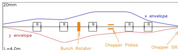
Figure 2: Beam envelopes for the initial MEBT section. The chopper plates are positioned after the third quadrupole where the 'x' divergence is very small. The chopper slits are positioned close to the stripping foil where the beam is focussed to a double waist.
