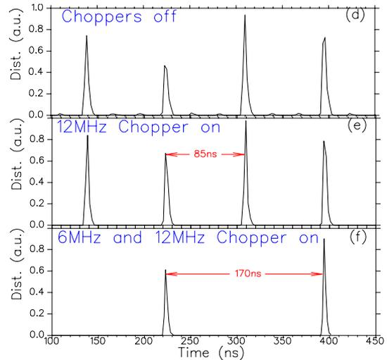
Figure 5: (a) Output time structure from the RFQ is shown in (a). The Mode A 11.8 MHz chopper plate produces a 85 ns time structure shown in (b). In Mode B the 5.9 MHz field is combined with the 11.8 MHz deflection to generate the time structure given in (c).
