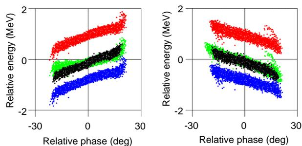
Figure 5: Energy spread reduction by sc bunch rotation cavities. Black dots: 'control' bunch, Green, red, blue dots:  $+3$  MeV,  $+6^\circ$ ,  $-2$  MeV &  $-4^\circ$  displacement at linac end
