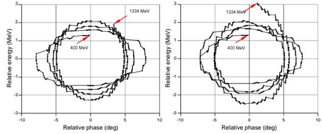
Figure 2: Synchrotron oscillation along the sc linac for initial +1.3 MeV displacement. Left: no RF errors, Right: with RF errors
