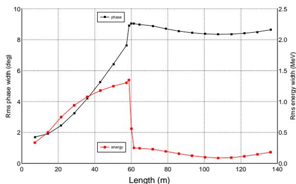
Figure 4: Rms phase width and energy spread along the linac to ring transferline
