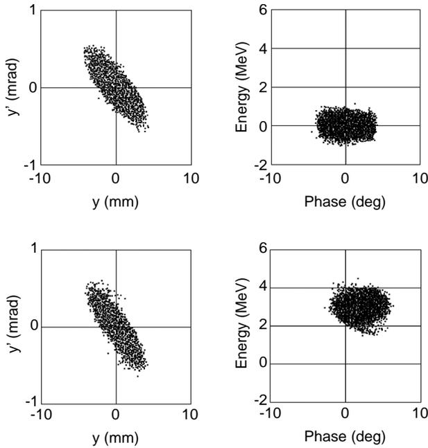
Figure 1: Horizontal and longitudinal phase space distributions at 1.334 GeV. Top: 'control' beam, Bottom: beam with RF errors and 1.3 MeV initial displacement
