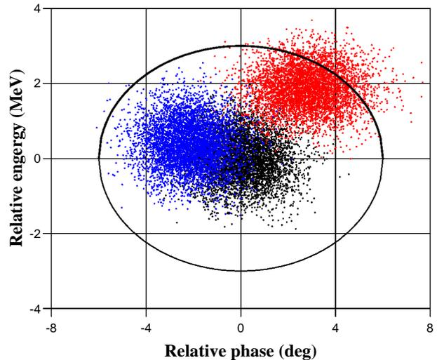
Figure 3: Scatter plot at 1.334 GeV due RF errors. Black dots: RF errors only, Red, blue dots: +1.3 MeV,  $+4^\circ$  initial displacement
