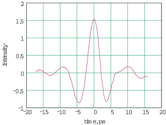
Figure 5: Autocorrelation function of the ELBE electron bunch measured with a Martin-Puplett interferometer.
