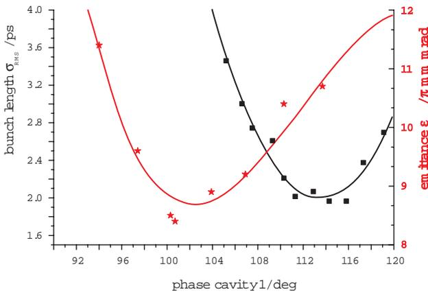
Figure 3: Bunch length and transverse emittance of the electron beam for varying first-cavity RF phase.
