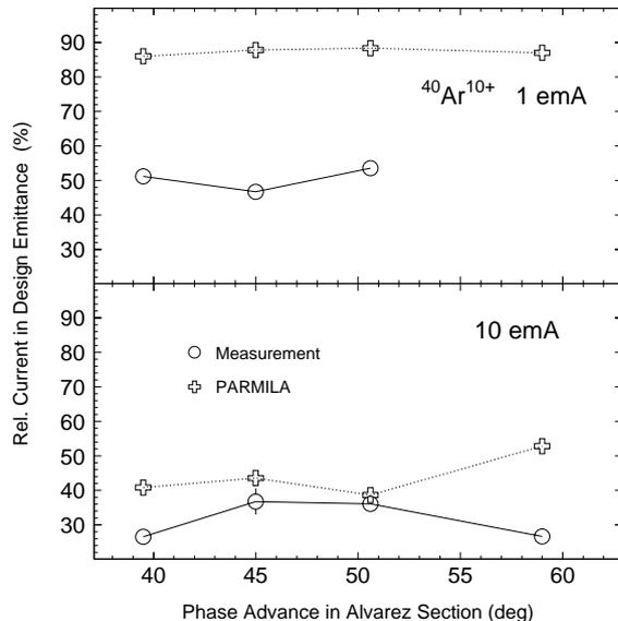
Figure 5: Current of  $\text{Ar}^{10+}$  (normalized to current at the slit-grid setup) in the transverse UNILAC design emittance after the Alvarez section as function of the transverse phase advance in the section for 1 emA (upper part) and 10 emA (lower part) after the stripper. The measured values are a lower limit of the brilliance.
