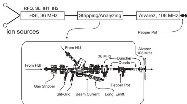
Figure 1: The Universal Linear Accelerator UNILAC.
