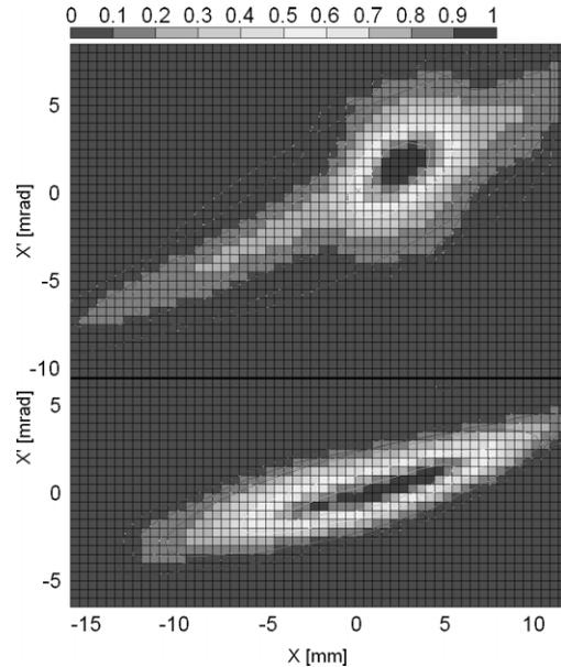
Figure 4: The horizontal phase space distributions measured with the pepper pot after the Alvarez section for an  $\text{Ar}^{10+}$  current of 10 emA and a transverse phase advance of  $39^\circ$  (upper part) and  $51^\circ$  (lower part). The measured transmissions were 78% and 92%, respectively.
