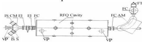
Fig.3 Layout of beam line for simul. acceleration
