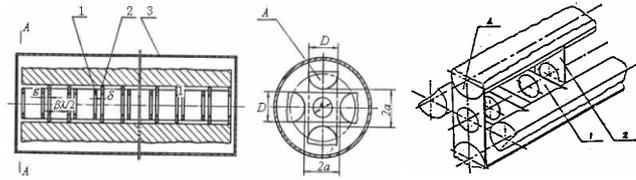
1&2 -diaphragms, 3 -cavity , 4 -quadrupole electrodes
