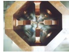
Fig. 10 RFQ cavity before brazing
