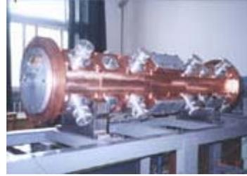
Fig.11 RFQ cavity after brazing
