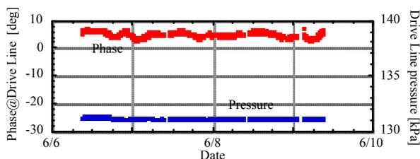
Fig. 4(b) N<sub>2</sub>-gas pressure and driveline phase drift (Feedback on)
