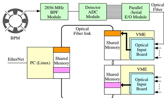
Fig.5 Block diagram of BPM data acquisition system
