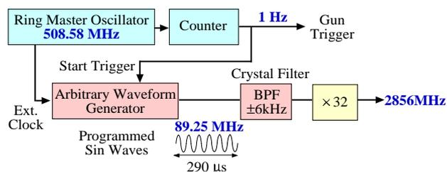
Fig. 1 Block diagram of RF reference generator.
