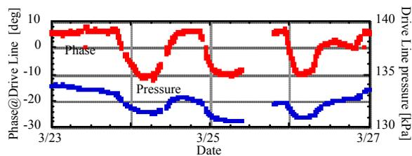
Fig. 4(a) N<sub>2</sub>-gas pressure and driveline phase drift (Feedback off)
