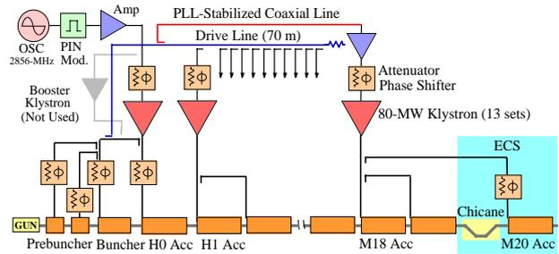
Fig.3 Diagram of improved RF
