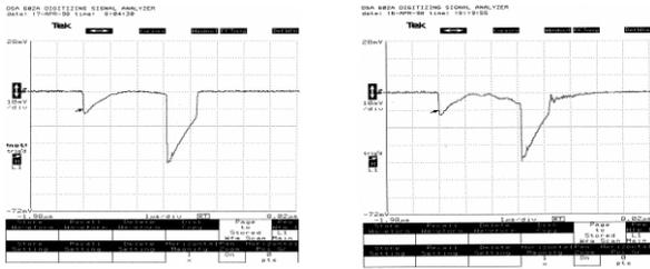
Figure 1: The RF waveform of pulse compressor output power; within temperature control of  $45\pm 0.1$  °C (left) and beyond temperature control of  $45\pm 0.5$  °C (right)[2]
