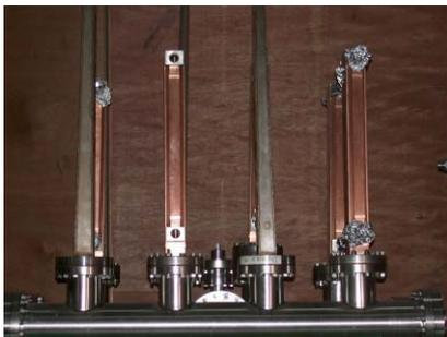
Figure 3: SiC loads and water-cooled RF loads under vacuum processing
