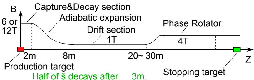
Fig. 2 Magnetic field distribution for PRISM/L
