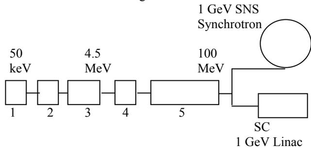
Figure 1. General schematics of the 100 MeV linac
