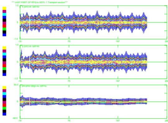
Figure 4. Beam transmission through first 22 tanks of the 100 MeV SDTL; Top x vs cell no; middle y vs cell no and bottom  $W-W_s$  vs cell no.
