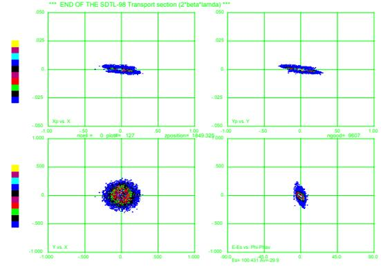
Figure 6. Beam phase space at the exit of the 98<sup>th</sup> tank of SDTL Top left  $x'$  vs  $x$ , top right  $y'$  vs  $y$ , bottom left  $y$  vs  $x$  and bottom right  $E-E_s$  vs  $\phi-\phi_s$
