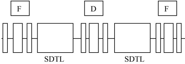
Figure 3. One period of the SDTL focusing lattice
