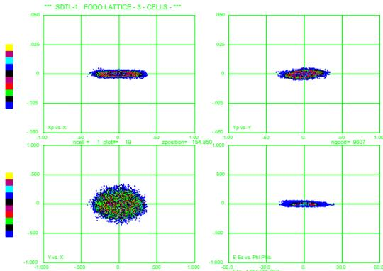
Figure 5. Beam phase space at the beginning of the MEBT Top left  $x'$  vs  $x$ , top right  $y'$  vs  $y$ , bottom left  $y$  vs  $x$  and bottom right  $W-W_s$  vs  $\phi-\phi_s$
