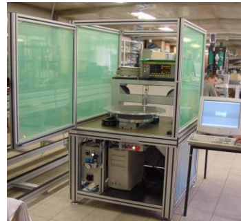
Figure 2: Setup for quality control of niobium sheet material for SNS
