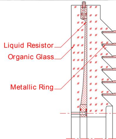
Figure 3: Photo(upper) and schematics(lower) of Radial Insulator
