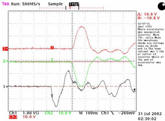
Figure 5: Anode voltage(upper) and cathode voltage(middle)
