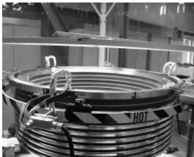
Figure 3 - Installation of Field Shapers
