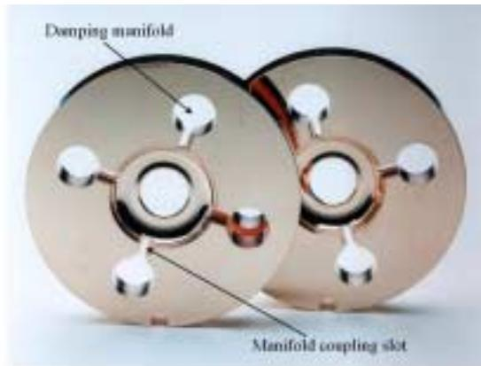
Figure 1: Two cells of NLC Structure RDDS1.
