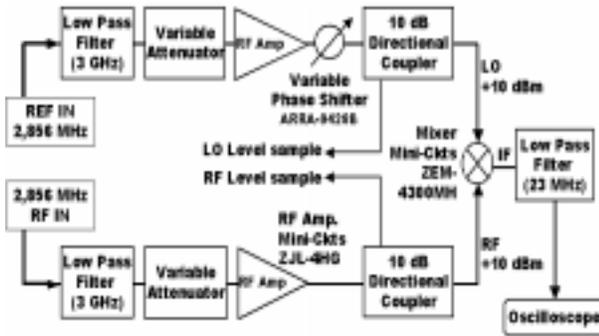
Figure 2: Block diagram of phase stability test unit.
