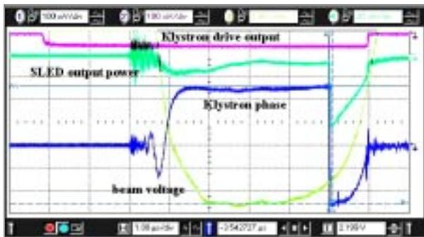
Figure 5: L2 before modulator trigger adjustments.
