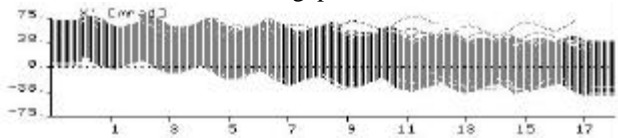
Fig. 10: Simulation of the beam bending by the multigap funnel deflector.
