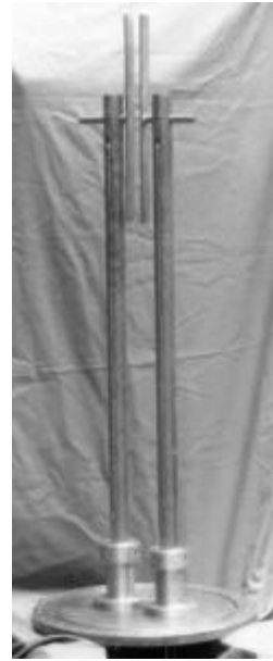
Fig. 5: Figure of the singlegap funnel deflector. The deflector discs are mounted at water-cooled stems. The length is about 2 m.
