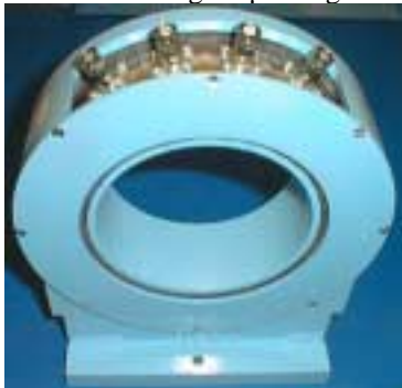
Figure 4. Bergoz ACCTs are installed with additional external magnetic-field shielding.
