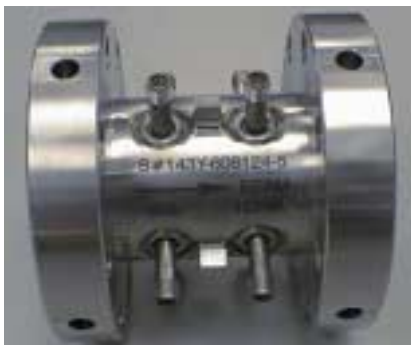
Figure 5. All of the BPMs have a sensitivity of 2.170 \pm 0.005 dB/mm and offsets < \pm 0.5 dB.
