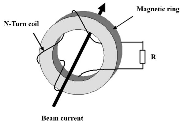
Figure 1: Beam current transformer schematic.
