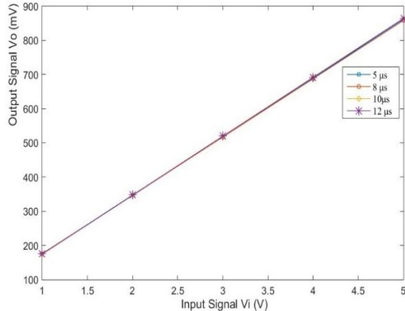
Figure 6: Vo vs. Vi fitted lines at different pulse widths.
