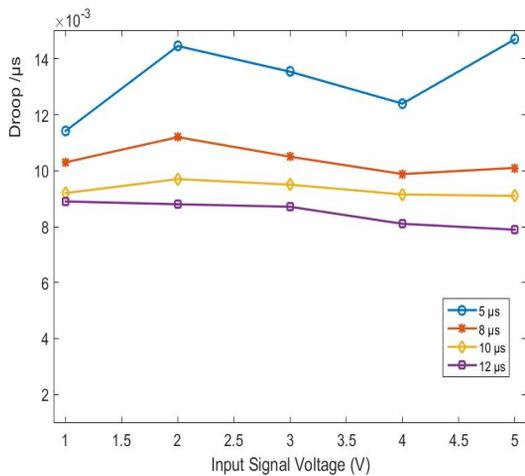
Figure 7: Curves of the droop at different pulse widths.
