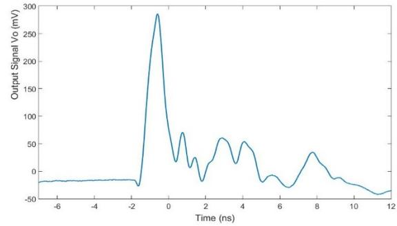
Figure 8: Waveform of a 1 ns short pulse.
