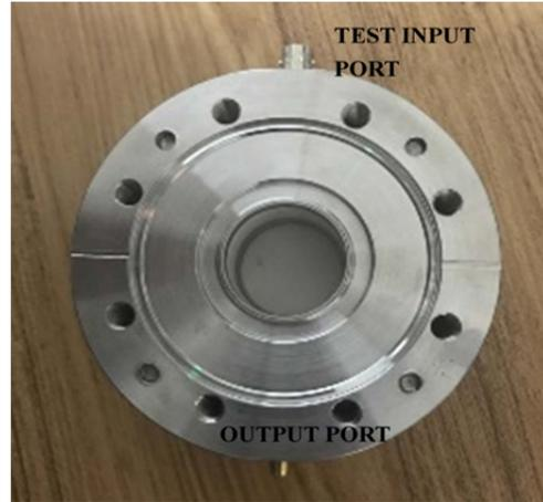
Figure 4: Picture of the beam current transformer.
