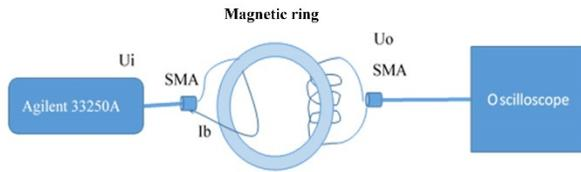
Figure 2: Block diagram of the magnetic ring test system.
