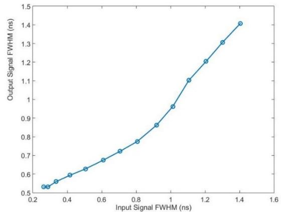
Figure 10: Curve of the inaction pulse FWHM with the input pulse FWHM.
