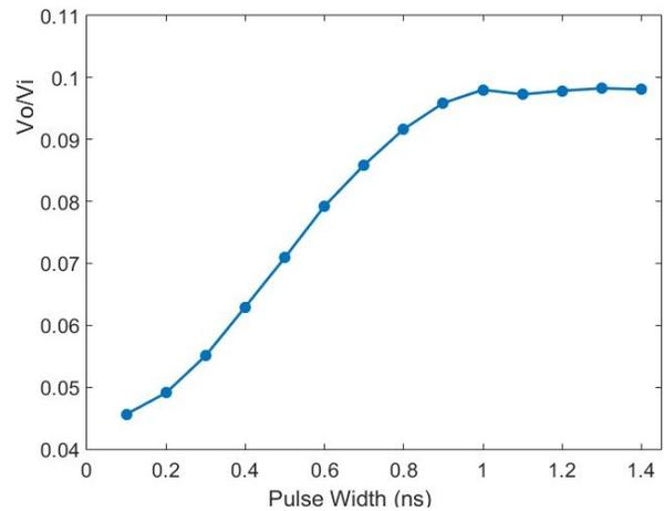
Figure 9: Curve of the ratio of output and input signal voltage with the ideal pulse width.
