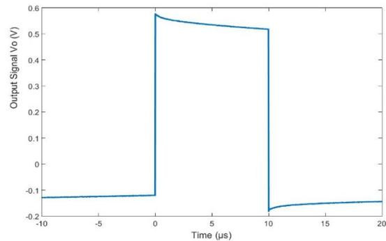
Figure 5: Waveform of a 10 µs pulse.
