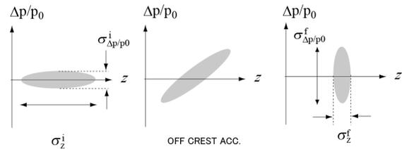
Figure 1: Schematic figure of longitudinal phase space in 1<sup>st</sup> order at bunch compression.
