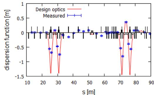
Figure 7: Dispersion function of the design optics of S2E simulation and measured one at energy recovery operation. The error bar is corresponding to 0.2 mm of BPM measurement.
