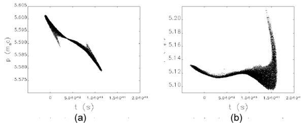
Figure 4: Longitudinal phase space of (a) entrance of the main linac before full acceleration (switching point) and (b) exit of the main linac after energy recovery.
