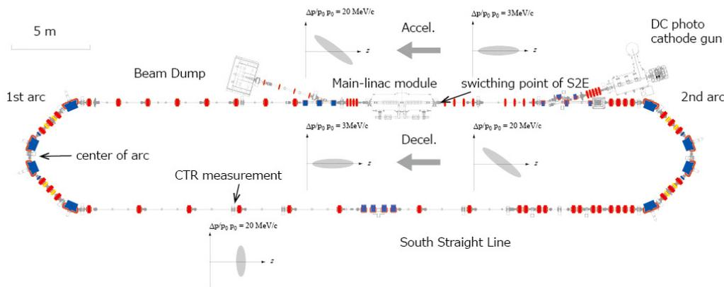
Figure 2: Schematic figures of longitudinal phase space of bunch compression and energy recovery in cERL. Simulation code used in start-to-end simulation is switched from GPT to elegant at the switching point.
