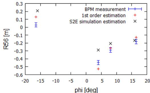
Figure 6: Relationship between RF phase and  $R_{56}$  of the first arc. The sign of  $R_{56}$  is opposite to the definition of ELEGANT.
