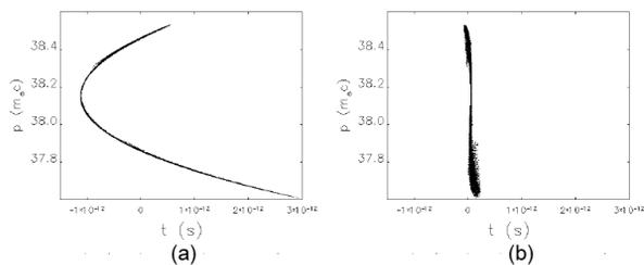
Figure 3: Longitudinal phase space at the CTR measurement system. (a) SX is off,  $\sigma_t = 670$  fs (b) SX is optimized,  $\sigma_t = 26$  fs.
