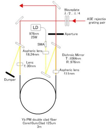
Figure 9: Double clad fiber amplifier by 1064 nm
