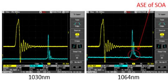
Figure 7: The pulse shape after the SOA
