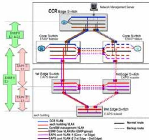
Fig.3 Protocol Configuration for Redundancy of network
