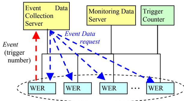
Fig.4 Configuration of WER Acquisition
