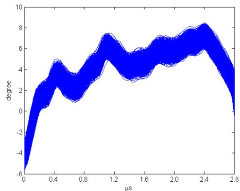
Figure 6: Interpulse phase shift of klystron forward signal
