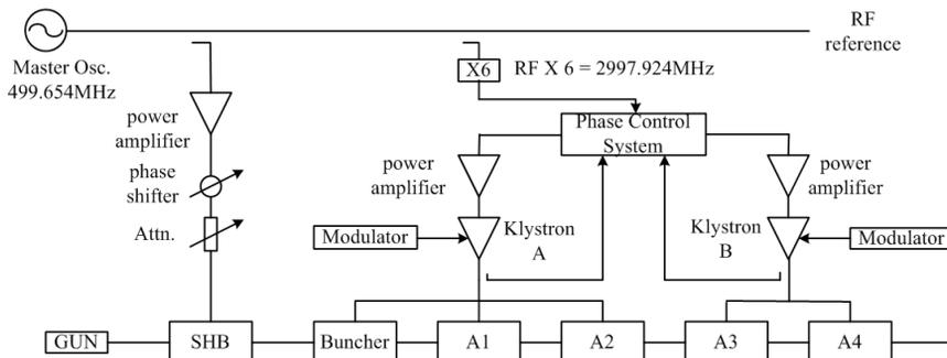
Figure 1: The layout of SSRF LINAC
