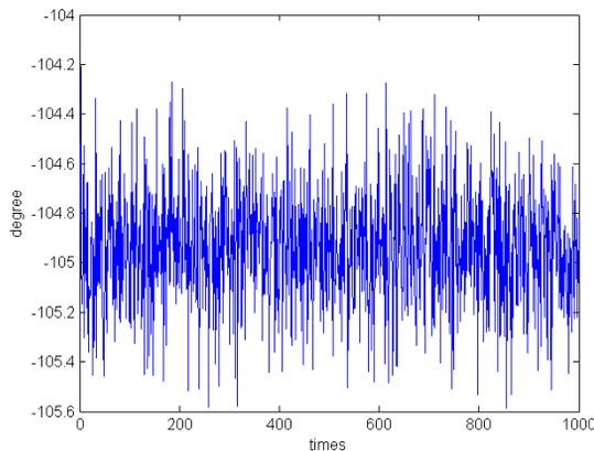
Figure 5: Background noise of phase control system
