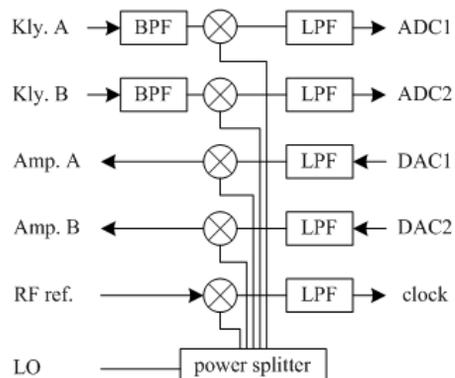
Figure 3: Layout of RF front-end
