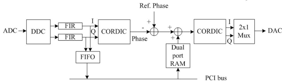
Figure 4: Layout of one channel in FPGA
