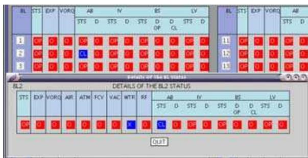
Fig.4 A screen shot of an operator console for emergency interlocks and summary status display for the beamline status
