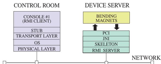
Figure 1: Simplified block diagram of a console and a device server using RMI communication for the 1.8GeV Synchrotron Radiation Source at TRSF
