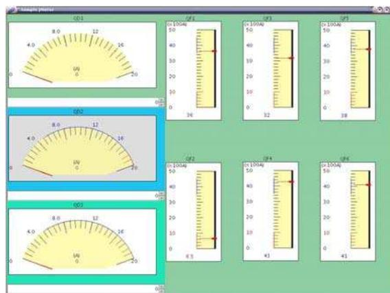
Fig. 3. screen shot of an operator console for quadruple magnets and some focusing/defocusing magnets.
