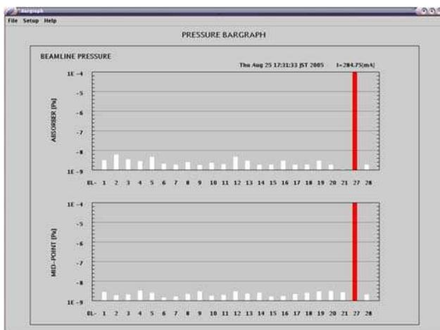
Fig.5 A screen shot of a console display for ultra-high vacuum of fifty beamlines
