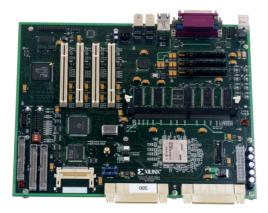
The development software supports several embedded operating systems, including VxWorks, LINUX, and QNX. The RHIC control system typically runs on VxWorks. Therefore efforts focused on evaluating the possibility of running RHIC controls software on the ML310 using VxWorks.
