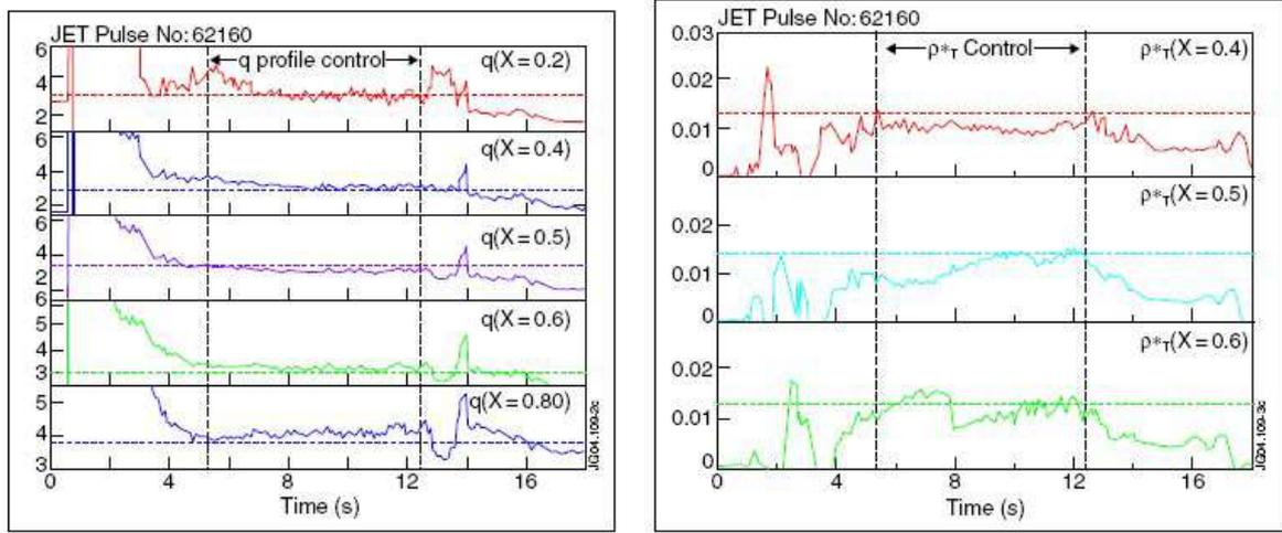
Figure 1: Time evolution of the measured and requested  $q$  values (a) at 5 radii and  $\rho^*_{Te}$  values (b) at 3 radii for a controlled pulse (Pulse No: 62160  $B_T = 3T$   $I_p = 1.7MA$ , current flat top starts at 4 s. Dashed lines are set point  $q$  and  $\rho^*_{Te}$  values. Control starts at 5.5 s and stops at 12.3 s.
