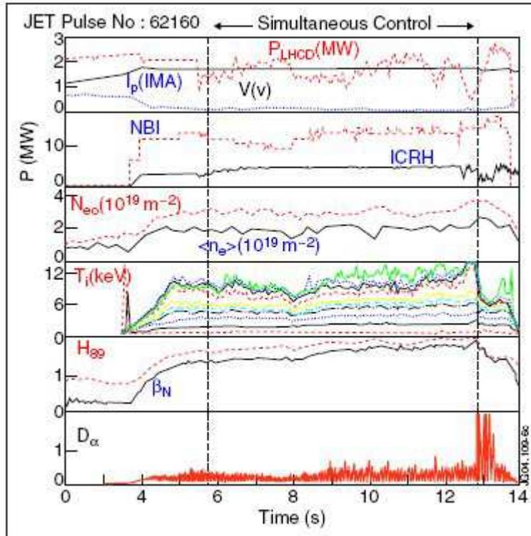
Figure 2: Time evolution of the LHCD, ICRH, NBI power waveforms, loop voltage, plasma current, central and mean density,  $T_i$ ,  $H_{89}$ ,  $\beta_N$ ,  $D_\alpha$  of a controlled pulse (Pulse No: 62160,  $B_T = 3T$ ,  $I_p = 1.7MA$ ).
