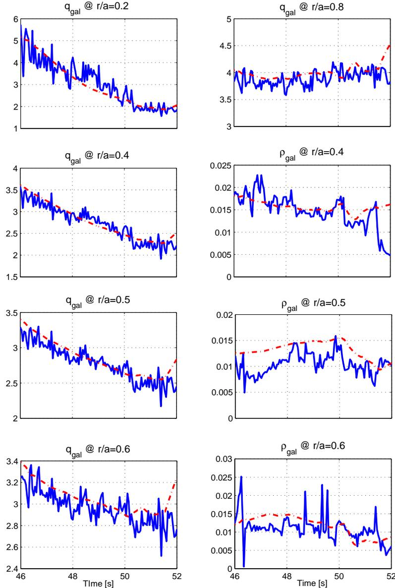
Figure 3: Time evolution of  $q$  and  $\rho^*_{Te}$  profiles as predicted by the identified model (1). The experimental traces are shown solid, the simulated traces dash-dotted. The simulation has been carried out in open-loop.
