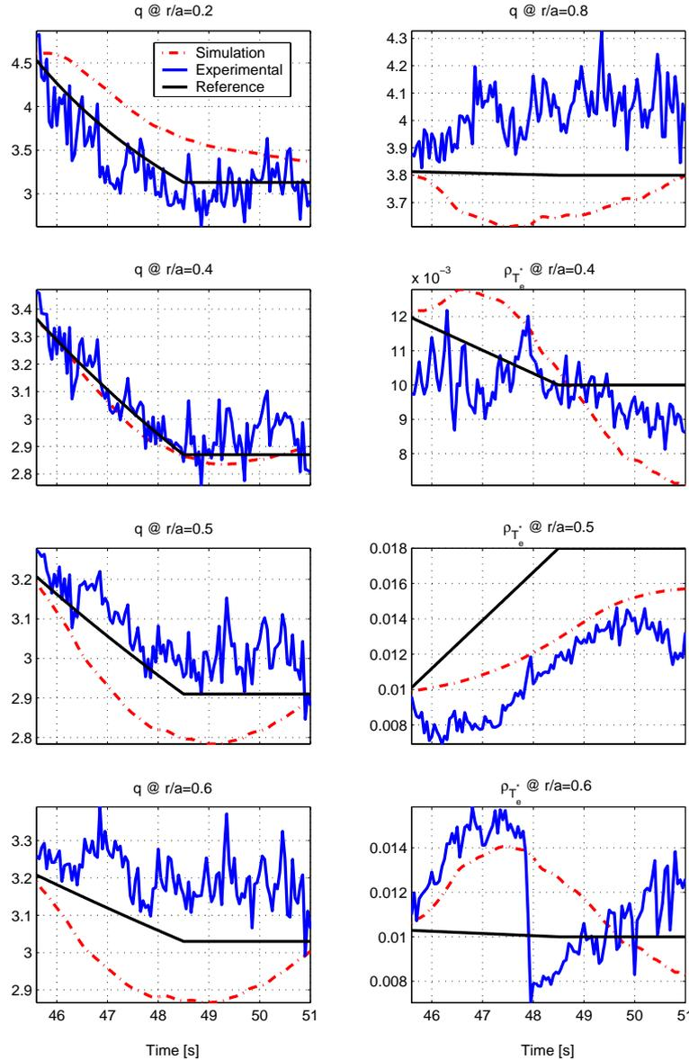
Figure 4: Time evolution of  $q$  and  $\rho^*_{Te}$  profiles as predicted by the identified model (1). The simulation has been carried out in closed-loop
