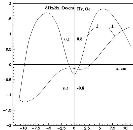
Figure 1: Magnetic field (1) and gradient (2) distributions introduced by the octupole winding.
