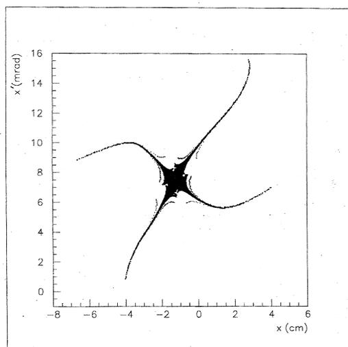
Figure 3: Computed phase plot of the electron resonance betatron oscillation.
