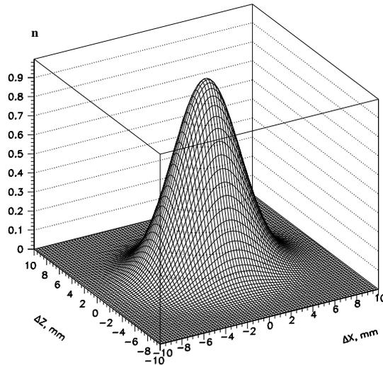
Figure 2: Two-dimensional distribution of electrons in the transverse cross-section of the beam.
