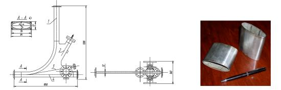
Figure 6: The bending magnet vacuum chamber for X-ray generator "NESTOR"
