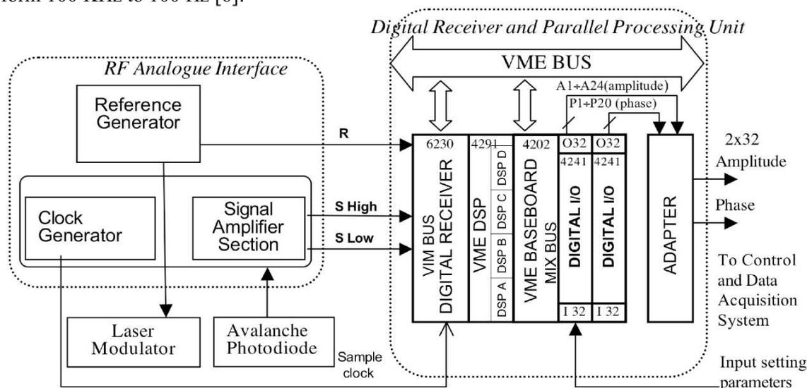
Figure 3: Radar Electronics (first implementation)
