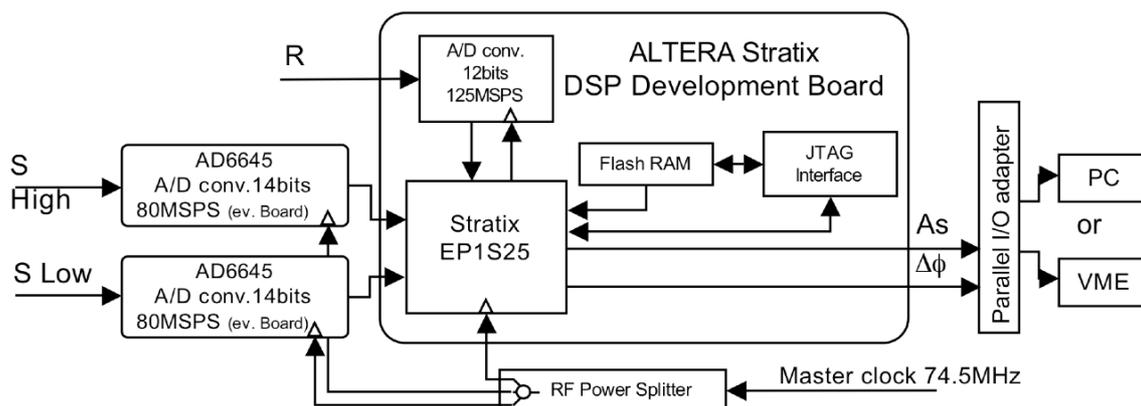
Figure 4: Radar Electronics (second implementation)
