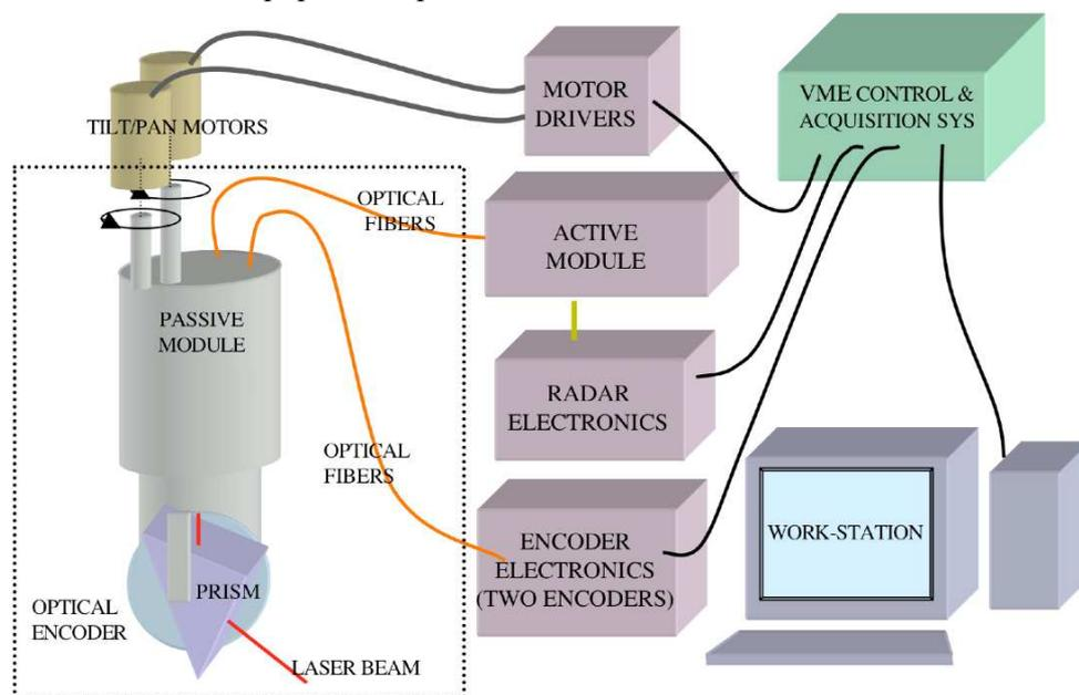
Figure 2: Control/acquisition/elaboration system layout
