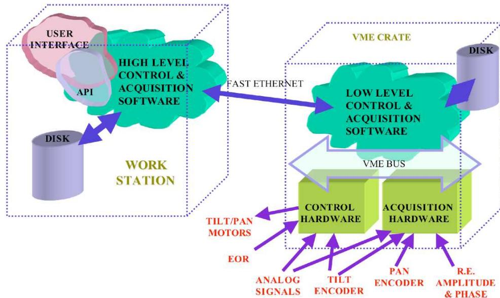
Figure 5: Control/acquisition system
