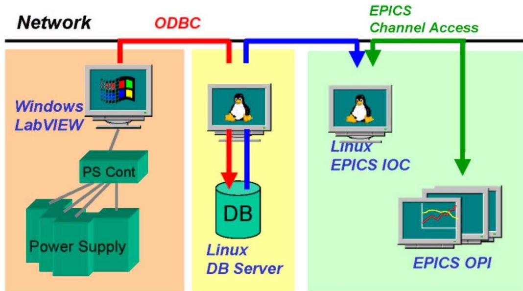
Figure 3: Magnet Power supply control system with relational databases
