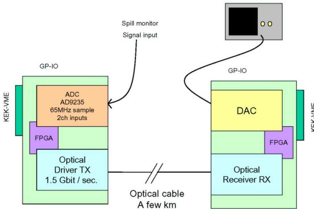
Figure 5: A schematic drawing of analog-to-optical signal transporter
