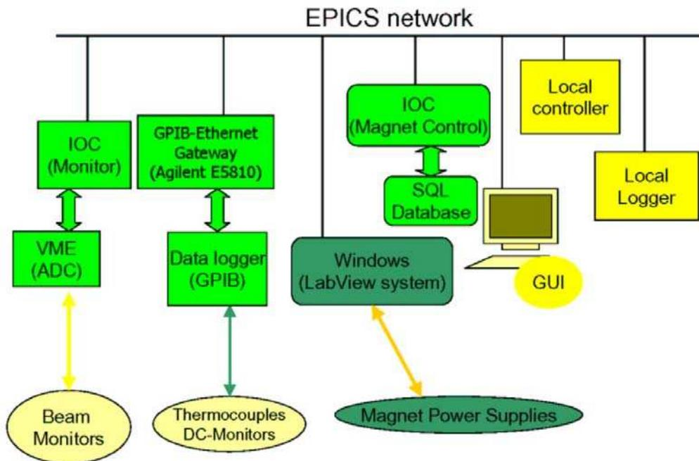
Figure 2: A schematic drawing of beam monitoring and magnet control system in HD-hall
